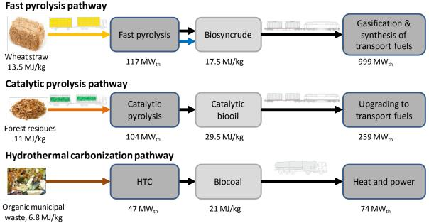
Figure 5: Feedstock, process steps and products for the three reference pathways along with the LHV of fuels (moisture, ash as received) and design (input) capacities of conversion plants.
