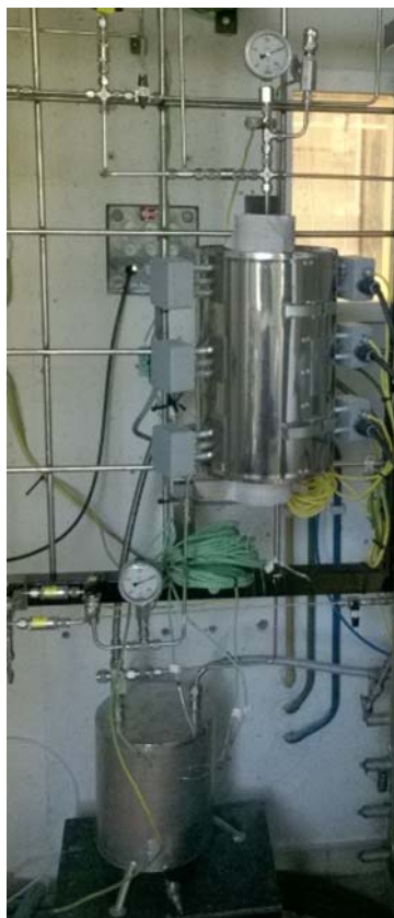
Figure 2. INTO equipment setup: Continuous tubular reactor (feed container and reactor oven with heating elements).
