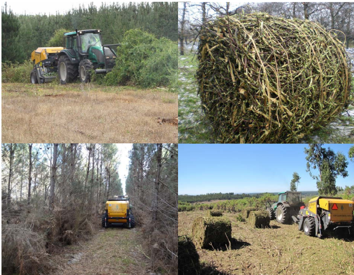
Figure 24: The BioBaler around the clock in invasive species removing, baling of fruit tree prunings, landscape protection and removal of understory vegetation. Copyright: Anderson Group co.
