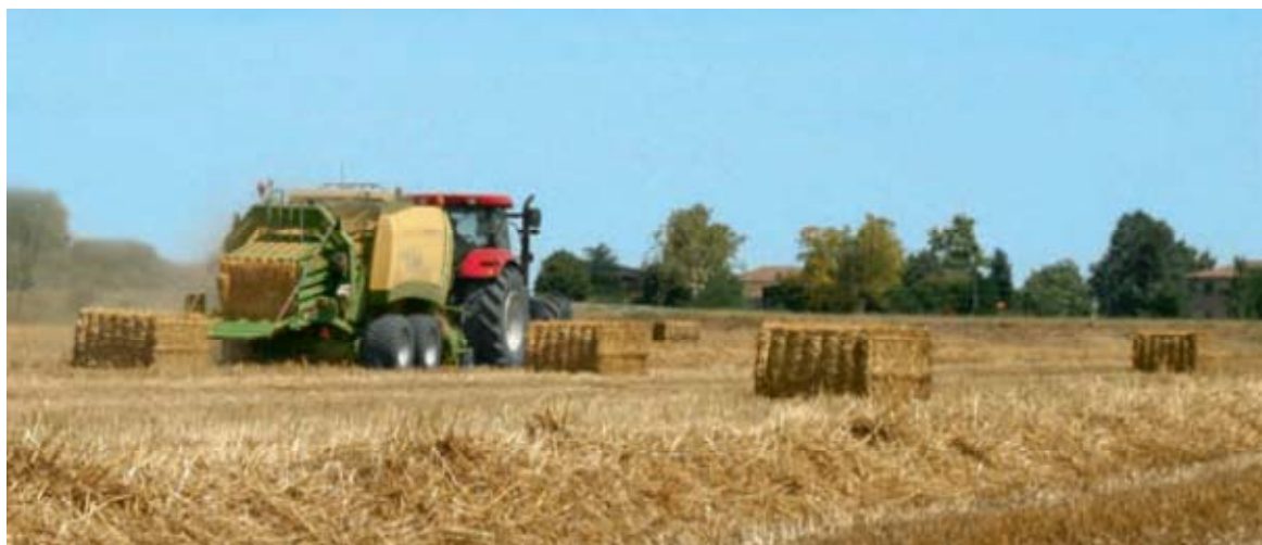
Figure 3: A large square baler of the 120 by 90 cm bale dimension and a high straw bale density of above 200 kg/m 3 as build by several manufacturers. Copyright: Krone
