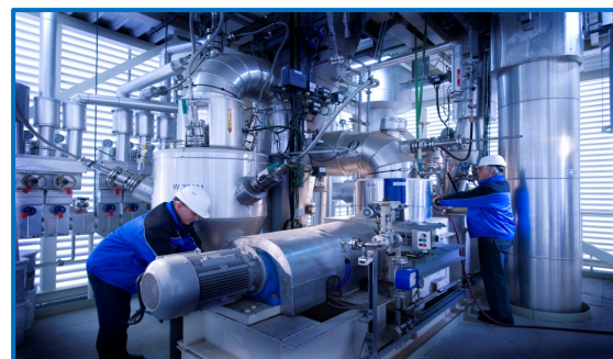
Top: b) FP yields of different types of biomass Bottom: c) FP reactor of 500 kg/h pilot plant.
