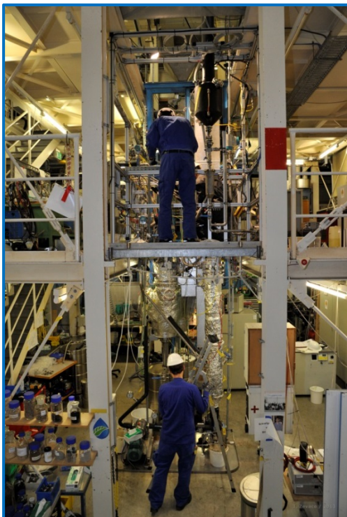
Figure 3: a) FP process development unit (10 kg/h) at KIT.
